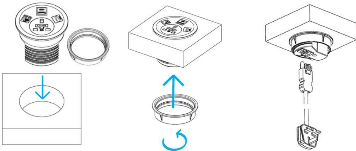
1. Remove the locking ring and place the module in the desk cut-out
