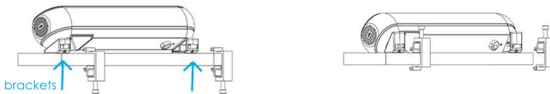
2. Use Allen key to fixate the module onto the desk
