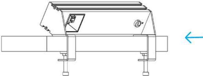
2. Use Allen key to fixate the module onto the desk
