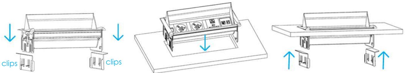
1. Lift the clips and slide the side fixators down.
