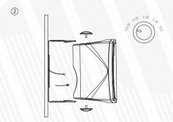
Place loudspeaker to the bracket and tighten by bracket knobs. Connect the wires. Set the desired loudspeaker power tap.
