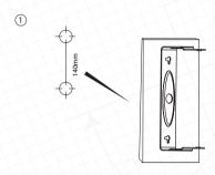
Drill holes according the drawing. Distance between the mounting points -140mm. Fix the loudspeaker bracket on the wall with fasteners suitable for your wall type.
