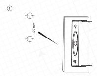
Drill holes according the drawing. Distance between the mounting points -170 mm. Fix the loudspeaker bracket on the wall with fasteners suitable for your wall type.
