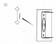
Drill holes according to the drawing.
