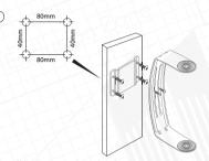
Drill holes according the drawing.
