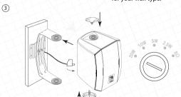
Place loudspeaker to the bracket and tighten by bracket knobs. Connect Euro block connector to socket. Set the desired loudspeaker power tap.
