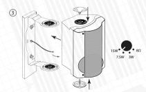
Place loudspeaker to the bracket and tighten by bracket knobs.
