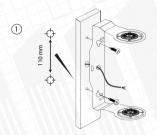
Drill holes according the drawing.
