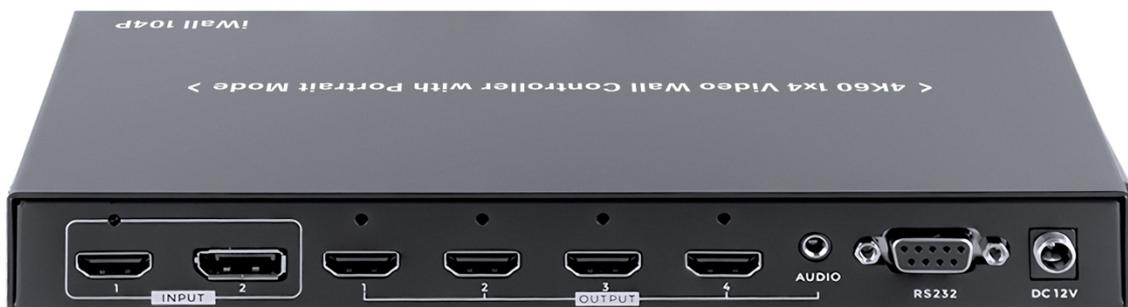
**INPUT:** #1 HDMI input, #2 DP (Not working simultaneously )
